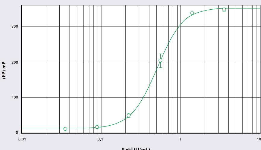
Lck kinase dilution curve with FAM-p34cdc2-derived peptide from 0.04 to 3.5 units/mL enzyme, read on Analyst HT (4-parameter curve fit).
