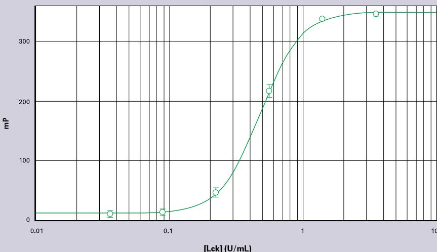
Lck kinase dilution curve with FAM-p34cdc2-derived peptide from 0.04 to 3.5 units/mL enzyme, read on SpectraMax M5 (4-parameter curve fit). Error bars here and on all subsequent graphs are standard deviations.
