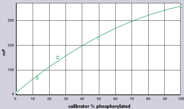
Calibration standard curve with FAM-p34cdc2-derived peptide and phosphopeptide, read on SpectraMax M5 (quadratic curve fit).
