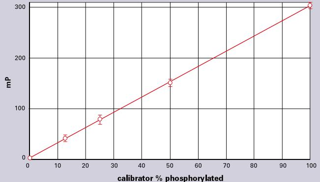
Calibration standard curve with TAMRA-p34cdc2-derived peptide and phosphopeptide, read on SpectraMax M5 (linear curve fit).
