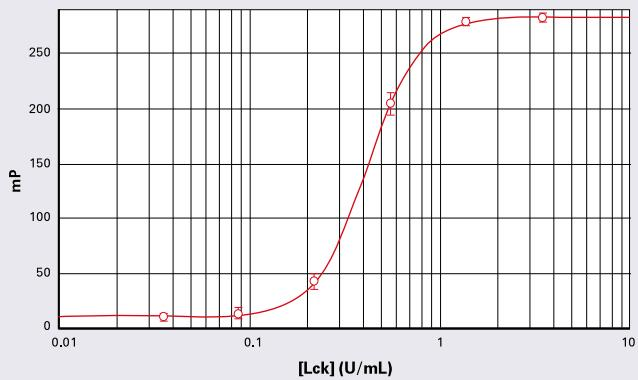
Lck kinase dilution curve with TAMRA-p34cdc2-derived peptide, read on SpectraMax M5 (4-parameter curve fit).
